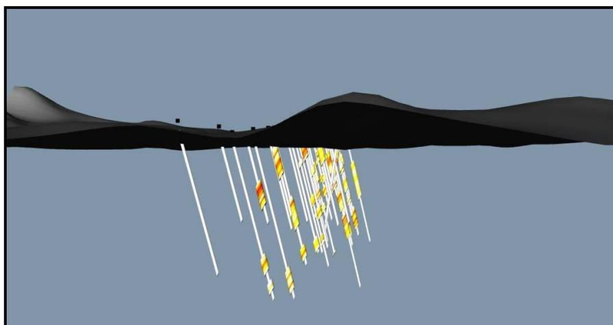
**Figure 4: 3D model of Skevi looking northwest with ASTER-DEM overlay. Coloured domains show where samples were collected. Hotter colours returned higher uranium values (i.e. red is >1000 ppm  $U_3O_8$ )**
